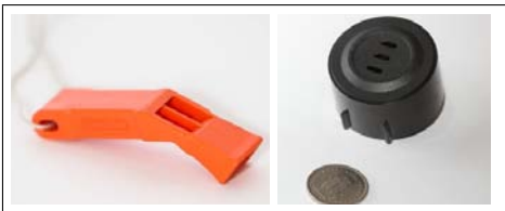
Fig. 5. (a) The safety whistle used in the experiment (commonly available in outdoor shops). It features two chambers, and emits two closely spaced, superimposed frequencies between 2kHz and 2.1 kHz. (b) A hand-held piezo alarm used in this work that emits a single frequency of 3.8 kHz.
