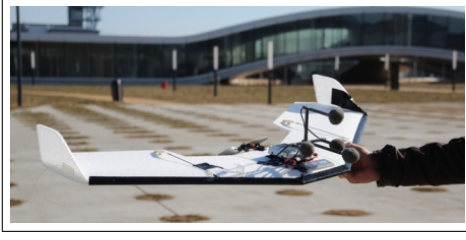
Fig. 4. Picture of the MAV platform [14] used for experimenting the proposed algorithm. Four microphones and an on-board digital sound recorder is used for recording sounds during flight.
