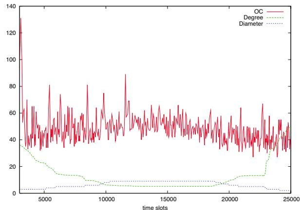
figure 8: Omnicast performance for 64 Nodes in a 2D configuration with slowly varying density (PDOR, schedule length 16 slots)
