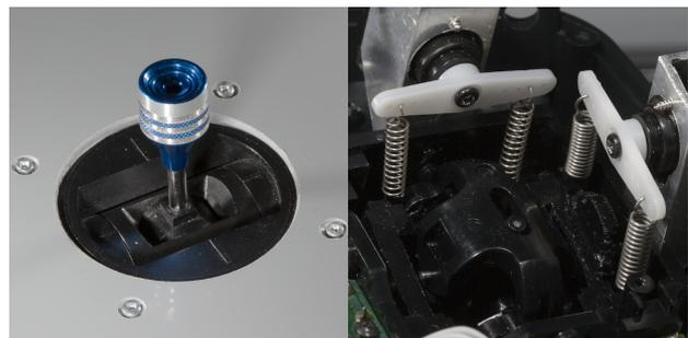
Figure 2: Control stick (left) equipped with haptic feedback servo motors (right)
